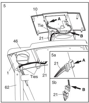
6. Set the Console (10) in the Console Base (46). Be careful to avoid pinching any wires. Insert the excess Wire Harness (21) into the large hole in the side of the right Handrail (1). Securely tighten the plastic ties on the bottom of the Console Base to prevent the Wire Harness from slipping. Cut off the ends of the plastic ties.
